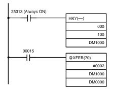
The hexadecimal key information that is input to IR 000 by HKY(—) is converted to hexadecimal and stored in words DM1000 and DM1001.
